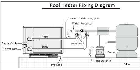
(Notice: The drawing is just for demonstration, and layout of the pipes is only for reference)
