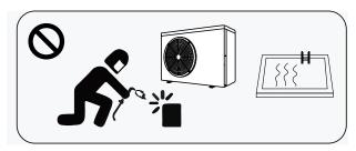
d. If a gas leak is detected during installation all work must stop and be reported to the heat pump supplier for service repair.
