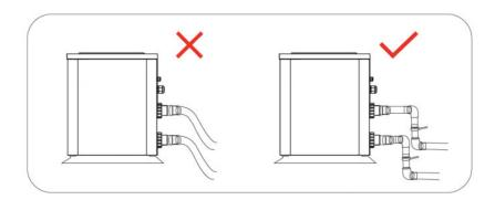
2.1.2. In order to guarantee the heating efficiency, the water pipe length should be  $\leq 10m$  between the pool and the heat pump.
