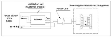
Note: The swimming pool heater must be earthed well.
